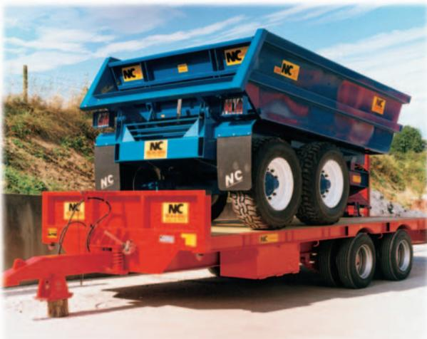
The careful positioning of the body pivot point ensures a maximum height of discharge, enabling the operator to stock pile top soil, or whatever with the minimum of ease. The NC Dump Trailer is designed wider and lower for better stability, hence making it easier to load with a rubber tyred or mini track digger, also the body can be scraped clean using a 6ft or 1.83m bucket.
